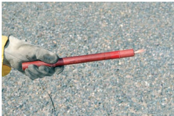
Fusees (shown in left photo) and flare launchers (shown in right photo) are lightweight and can be useful ignition devices when fuel or topography pose safety issues. Photos: National Wildfire Coordinating Group.
