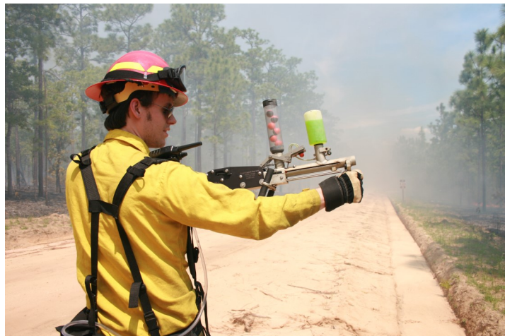
Hand-held DAID launchers allow prescribed burners to quickly ignite fire without entering potentially unsafe areas. Photo by David Godwin.
