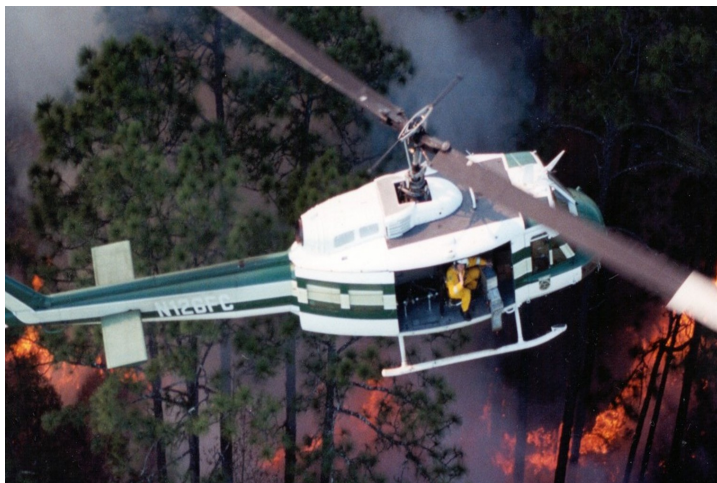
Aerial ignition systems can be used for large burn units or multiple small units, and generally allow for more rapid smoke dispersion than with ground-based devices. Photo by Georgia Department of Natural Resources.
