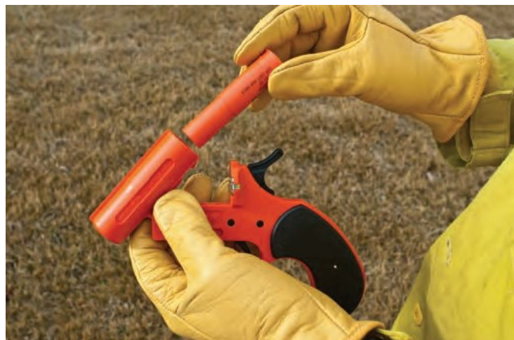
Fusees (shown in left photo) and flare launchers (shown in right photo) are lightweight and can be useful ignition devices when fuel or topography pose safety issues. Photos: National Wildfire Coordinating Group.
