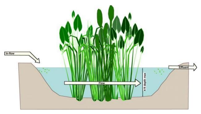
Fig 1. Diagram of a surface flow constructed wetland. Image by Dr. Sarah White (Oki and White, 2012).
