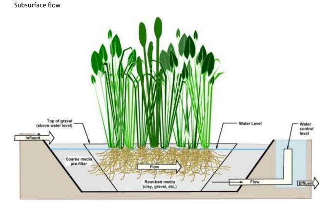
Fig 2. Diagram of a subsurface flow constructed wetland. Image by Dr. Sarah White (Oki and White, 2012).
