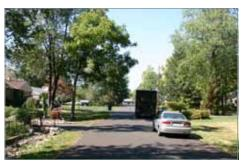
This 22- foot-wide street calms traffic, reduces impervious coverage, and allows service vehicles.
