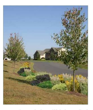
The swale along this road could be planted with a mixture of perennials. This would help slow runoff and provide greater infiltration of stormwater.
