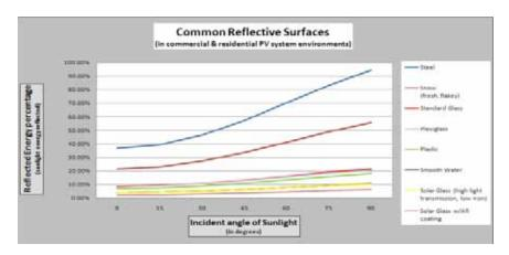
Figure 2.4: Common Reflective Surfaces and reflectance percentages.
