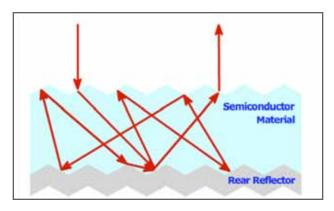
Figure 3.1: Light Trapping. More light energy is absorbed by the cell with each ensuing reflection of the initial light beam.
