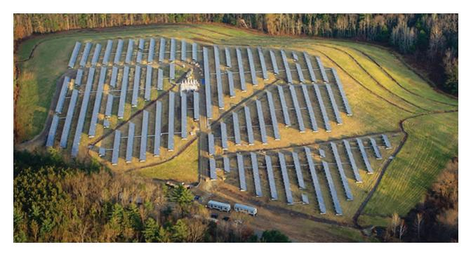
A 2.3 MW PV system on a capped landfill in Easthampton, Massachusetts
