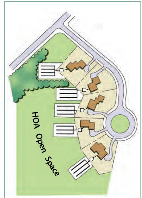
**Figure 21 Septic Systems in Common Open Space**
