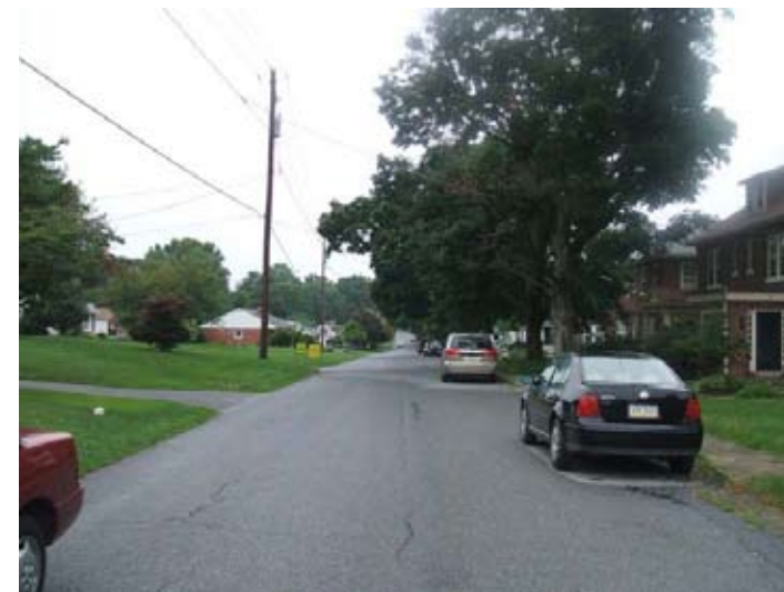
The cross section of Brandt Blvd. This two-way street had a very narrow cartway which helped to lower traffic speeds.
