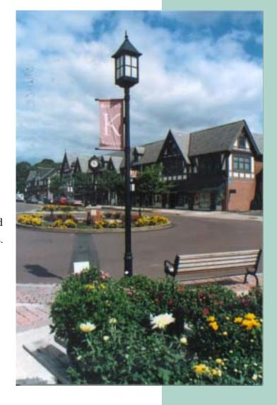
sections roundabouts can reduce traffic speeds to 15-20 mph and reduce crashes by 50-90 percent. Roundabouts are a popular and effective way to slow traffic, reduce through traffic, and improve the aesthetics of our communities.
